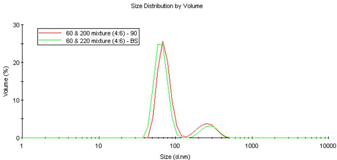
**Figure 3:** Volume weighted particle size distribution for a mixture of monodisperse 60 and 200 nm latexes, at a 4:6 volume ratio, measured at 90 and 173 degree scattering angles.
