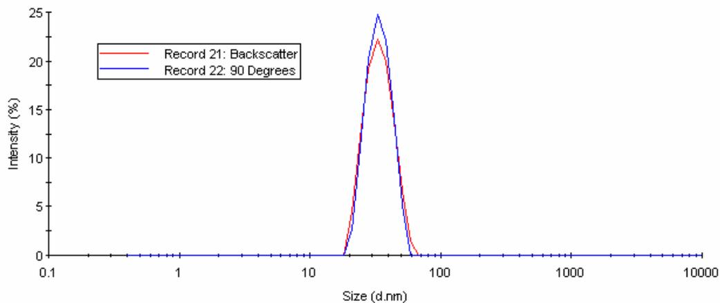
**Figure 1a:** Intensity particle size distributions measured at 90 and 173 degrees for a monodisperse 30 nm latex.
