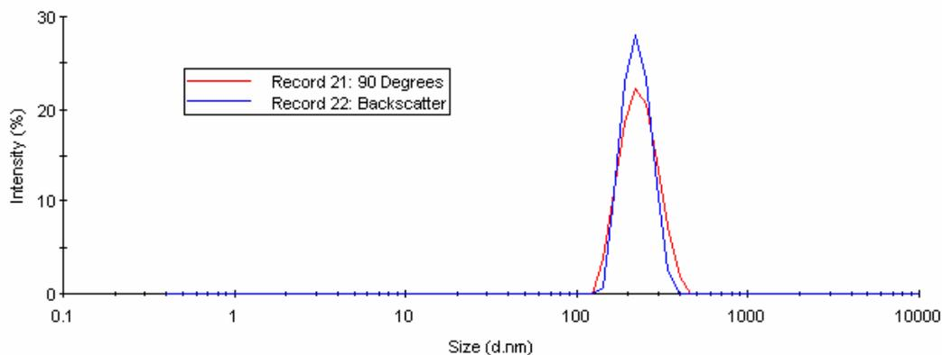
**Figure 1b:** Intensity particle size distributions measured at 90 and 173 degrees for a monodisperse 220 nm latex.
