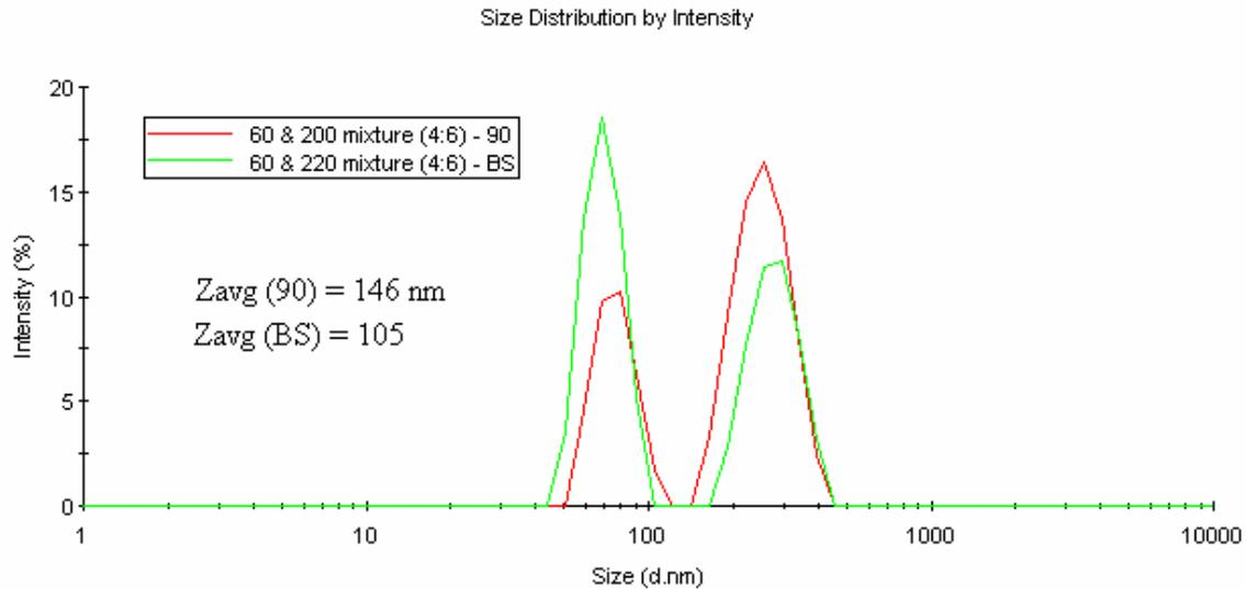
**Figure 2:** Intensity particle size distribution results for a mixture of monodisperse 60 and 200 nm latexes, at a 4:6 volume ratio, measured at 90 and 173 degree scattering angles.
